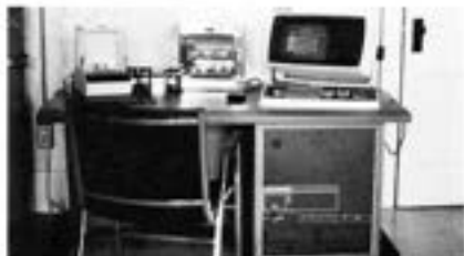
Fig 1 Micro-Coal 1 control console. MicroNova microcomputer is in cabinet at right, just above dual floppy disc drive. Interfacing circuitry and audio alarm are in upper section of cabinet. CRT displays main menu, allowing operator to choose laboratory functions. Balance at left corner of desk weighs samples of up to 30 g at accuracy to 0.0001 g. Pedal switch to left of CRT terminal strobes microcomputer for reading balance.
