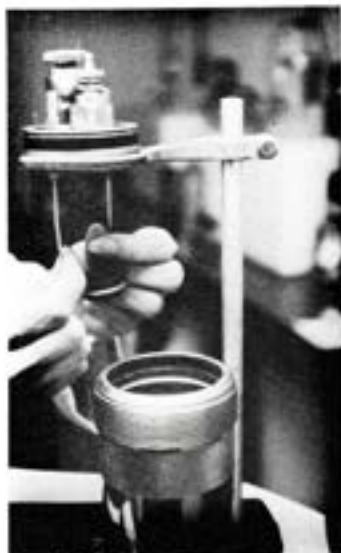
Preparation of the oxygen bomb in BTU determination—a far cry from bombs of earlier days.
