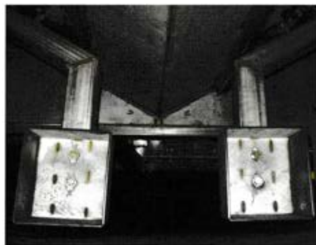
Figure 3. The MPS includes double sample scoops (Note: during operation, they alternate via a timer).
