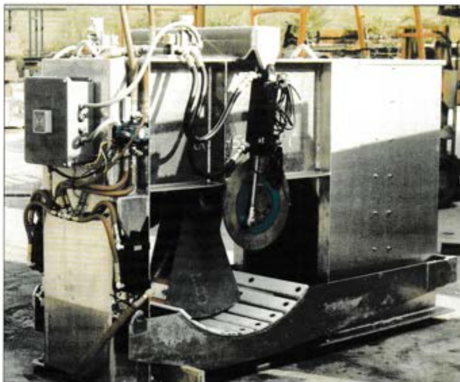
Figure 6. Support mechanism for shaping the conveyor belt to the required contour for precise sampling.
